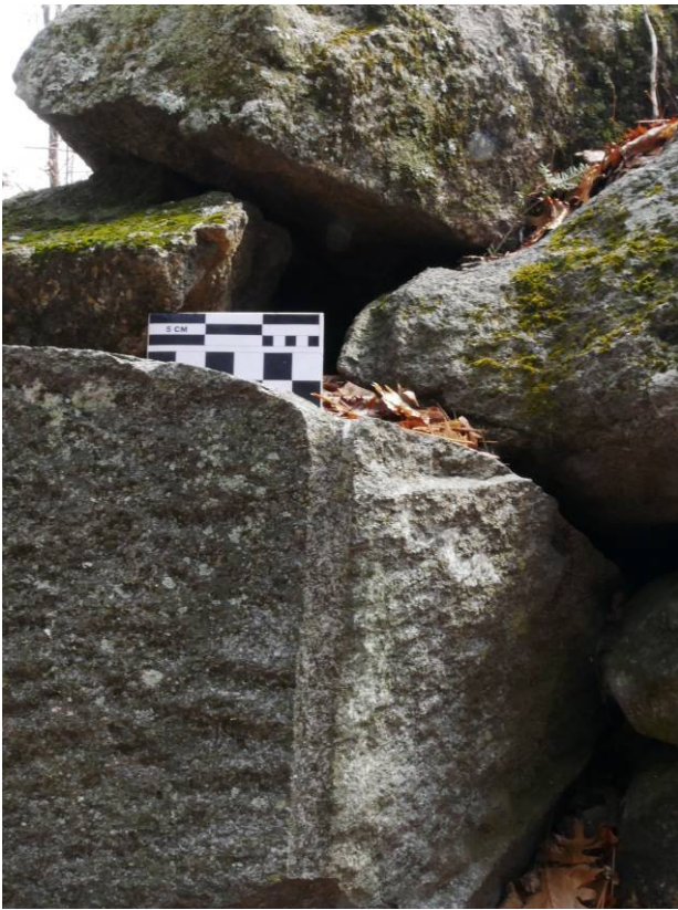
Figure 1 – Example of a 1 ½ inch diameter x 18 inch deep hole drilled into a field boulder to blow it apart with gun powder.
